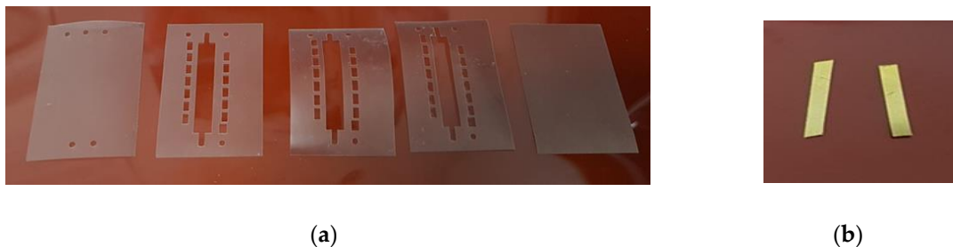
139 Figure 4. (a) Separate layers of PVC foil for inductor fabrication, (b) conductive segments for solenoid turns.
