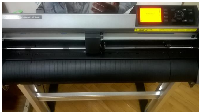
Fig. 2. Cutter for Xurographic techniques.
