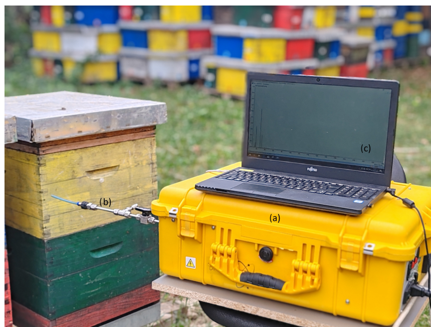
Figure 1. In-field system setup: (a) Portable membrane inlet mass spectrometer with (b) sampling probe and (c) laptop for acquisition and processing of the results.
