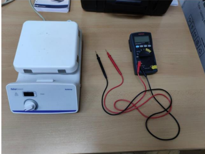
Fig. 2. Experimental setup for measuring the resistance of the sensor with increasing of the temperature
