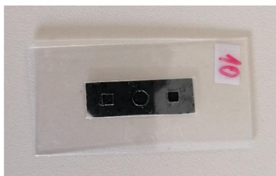
Figure 2. Fabricated microfluidic platform with MWCNTs-functionalized filter paper in the middle of the structure
