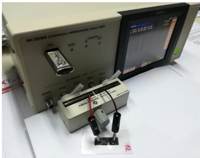
Figure 3. Experimental set-up for measuring electrical parameters of the proposed microfluidic platform
