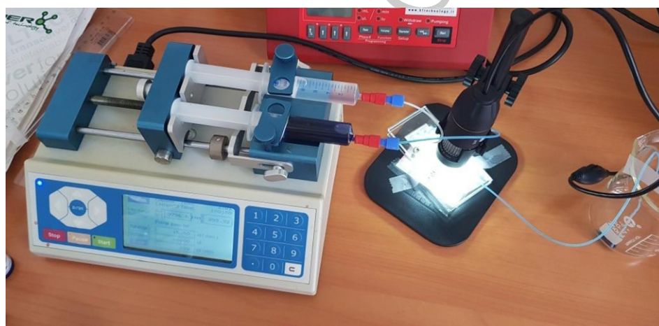
Fig. 2. Experimental setup employing syringe pump.
