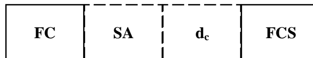
229 230 Figure 3: Wake-up beacon (WB). FC and FCS represent Frame Control and Frame Check Sequence fields, 231 respectively. 232
