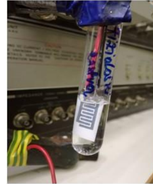
Fig. 4. Fabricated sensor on paper substrate.
